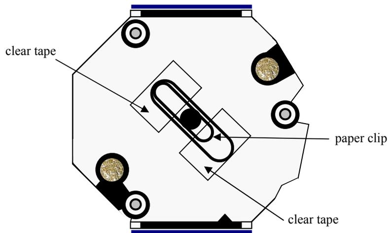
8. Inflate the balloon to maximum size and then deflate it at least five times to stretch it out. Poke the nozzle of the balloon through the paper clip and hole in the **science deck** with the pencil so it looks like the diagram below. Pull the balloon up so that the nozzle of the balloon lies flat against the **lander bottom**.
